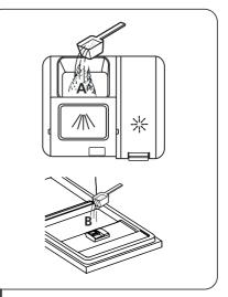
Add detergent into the larger cavity (A) for the main wash cycle . For better cleaning result, especially if you have very dirt items, pour a small amount of detergent onto the door. The additional detergent will activate during the pre-wash phase.
