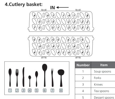
Information for comparability tests in accordance with EN60436 Capacity: 12 place settings Position of the upper basket: lower position Program: ECO Rinse aid setting: Max Softener setting: H3
