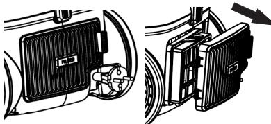
2. Remove the filter, clean it or replace it with a new one.
